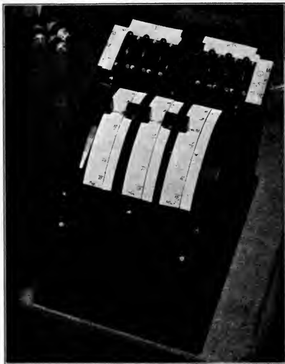
FIG. 4. The enhancement control unit of the stereophonic system provides both volume and frequency control at the discretion of the conductor.
